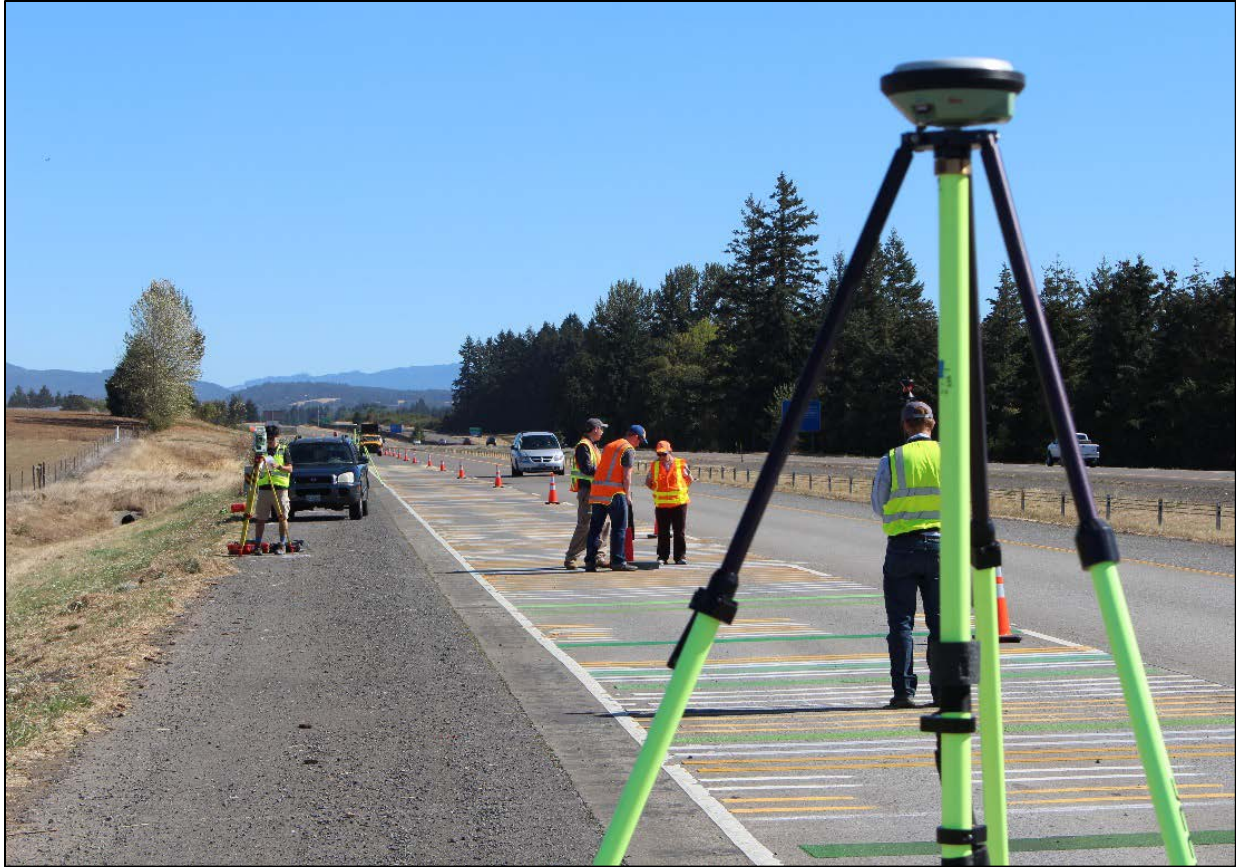
Figure 5.2: Acquisition of GNSS survey control data, retroreflectivity readings, and total station coordinates on locations of retroreflectivity readings.
