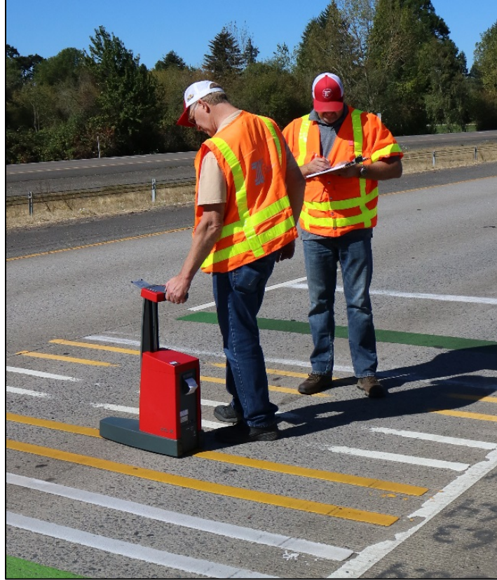
Figure 2.2: Retroreflectometer being used to measure retroreflectance of pavement markings on the Oregon Department of Transportation Testdeck.
