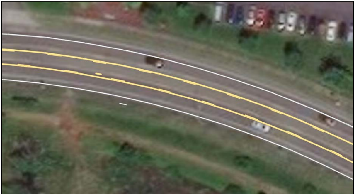
Figure 12.12: Example output of the stripeeditor.py script showing correct yellow and white stripes with transverse stripes removed. This data is the combination of 2 runs (clockwise and counter-clockwise) on the Oregon DOT Salem mobile lidar test course.
