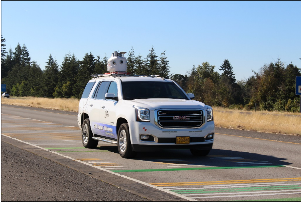
Figure 4.2: Oregon DOT's Leica Pegasus:Two mobile lidar system collecting data on the Testdeck.
